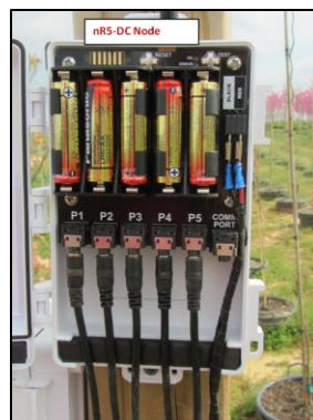
Fig 1. Inside of an nR5-DC node used for irrigation control. Solenoid wires can be seen to the right of the batteries [Lea-Cox & Belayneh, 2012].
